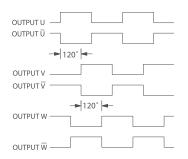
CW ROTATION OF SHAFT AS VIEWED LOOKING AT THE ENCODER FACE. NOTE: ALL DEGREE REFERENCES ARE ELECTRICAL DEGREES. WWEFORM SHOWN WITH OPTIONAL COMPLEMENTARY SIGNALS Ä, B, Ž FOR HV AND OD OUTPUTS ONLY.
